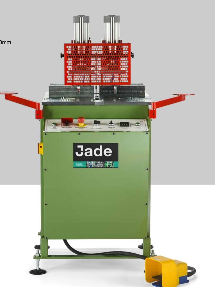
The CW225 UPVC Double Reverse Butt Welder, comes with two sets of fences allowing the fabricator to complete two butt welds in a single cycle. The CW225 is fitted with 0.2mm restriction knives, therefore achieving a perfect finish on both foiled and non-foiled products. Due to the unique variable angle fences, the CW225 also has the capability of welding cills up to 225mm wide when cut at 45°.
