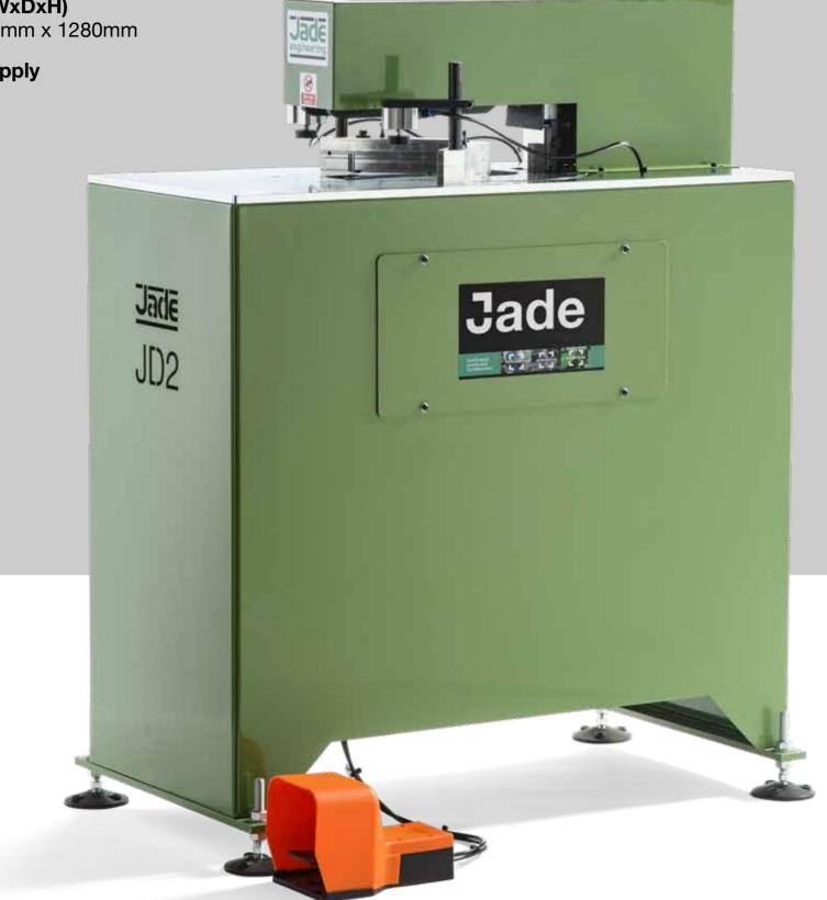
The JD2 Groover allows the fabricator to clean the excess weld sprue on the top and bottom faces of either reverse butt or corner welds. The JD2 comes equipped with adjustable back fences which can be easily rotated from 180° to 60°. There is also a fence setting which allows the user to clean cruciform welded joints. The JD2 is a floor standing machine operated by foot pedal and comes complete with top and bottom knives to customer's specification.
