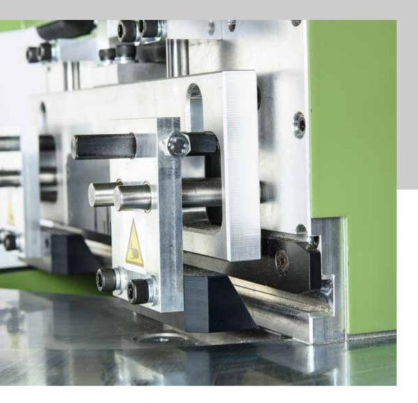
The JS250 CNC is an Up-Cut saw with a blade diameter of 250mm.
