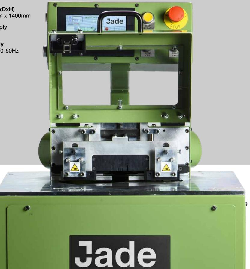
The JS250 CNC Bead Saw is the successor to the very popular JS250P. Now available with a 7" touch screen for ease of use, the JS250 CNC comes with a new clamping arrangement which includes an adjustable glass simulator where you can cut multiple types of beads without the need of changing support blocks.
